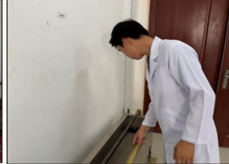
Ductility Test of Bituminous Material
