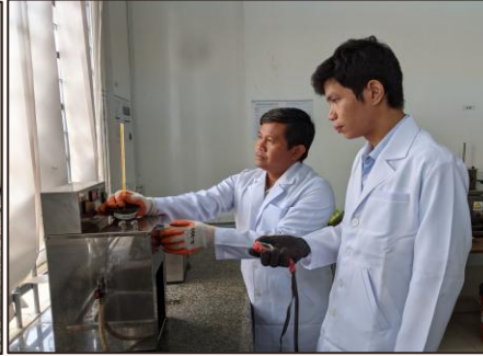
Viscosity Test of Bituminous Material
