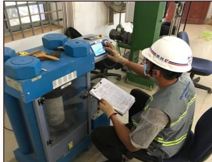
Compressive Strength Test of Concrete
