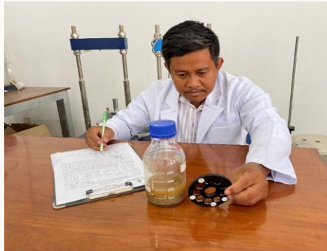
Organic Impurities of Fine Aggregates for Concrete
